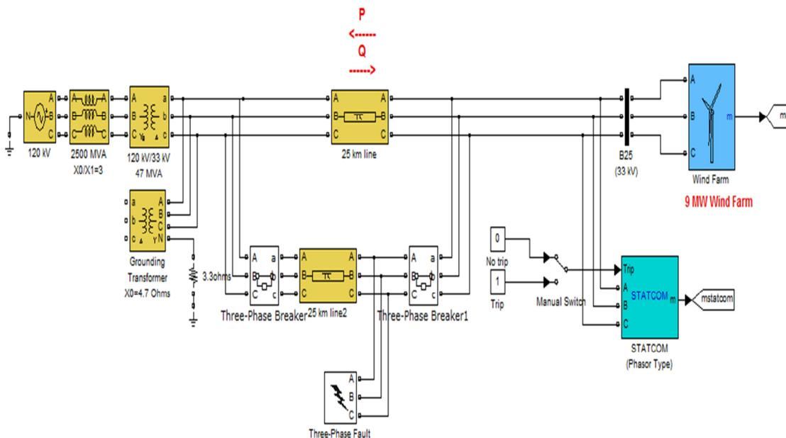
Fig 1. System Model with STATCOM
