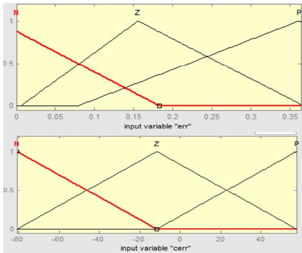
Fig 7. Fuzzy Set for input and their corresponding membership functions
