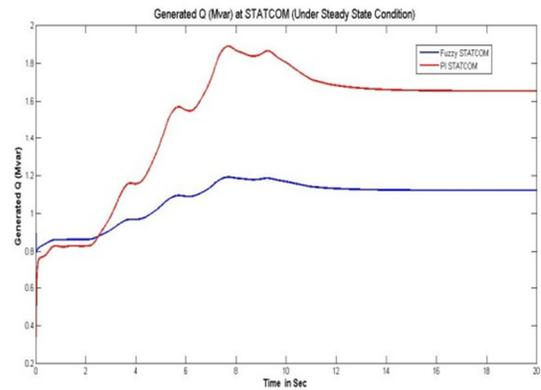
Fig 12. Generated Q (Mvar) at STATCOM under steady state condition
