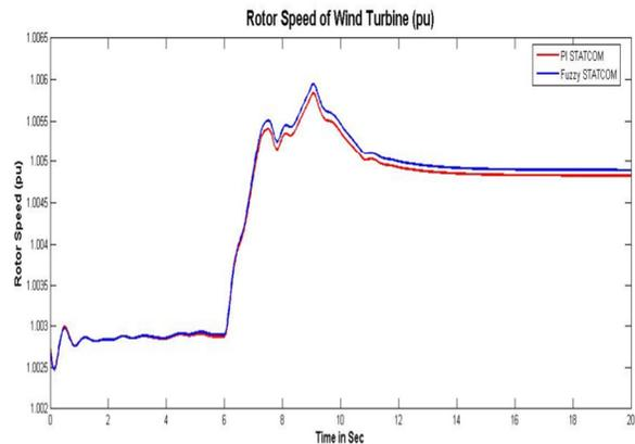
Fig 12. Rotor speed of wind turbine (in p.u) under steady state condition
