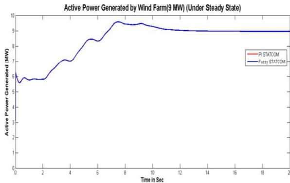
Fig 10. Active Power Demand under steady state condition
