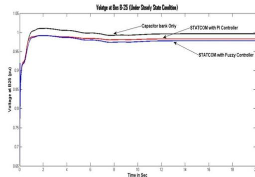
Fig 9. Voltage at Bus B-25 under steady state condition
