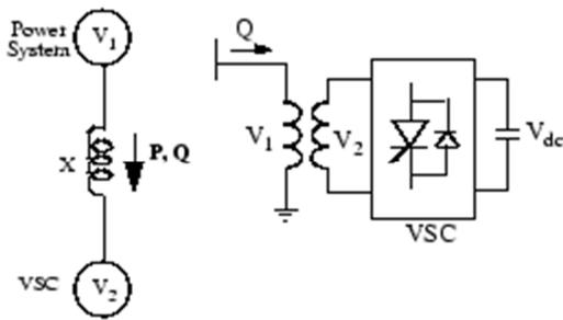
Fig 2. Single line diagram of STATCOM
