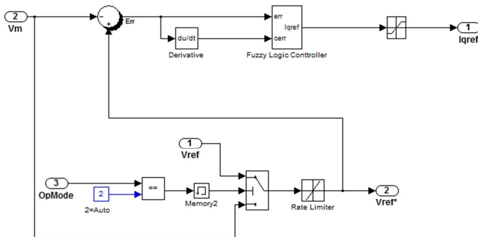
Fig 5. Fuzzy Logic Controller connected in STATCOM
