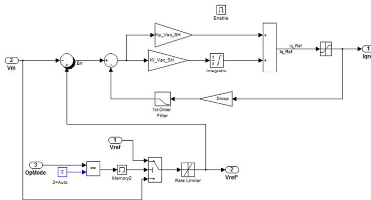
Fig 4. PI Controller connected in STATCOM
