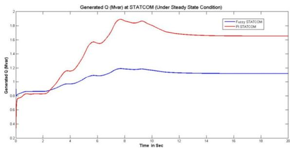
Fig 11. Reactive Power Demand under steady state condition
