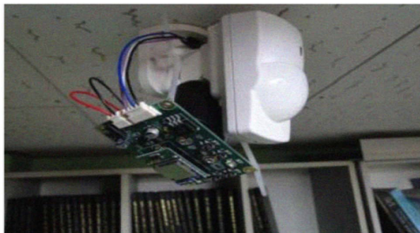
2c- ZED installation with PIR sensor
