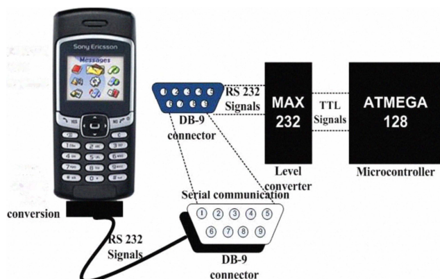
Figure 3: Serial Communication and Level Conversion between T290i and MCV
